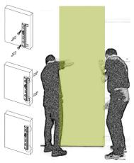
Put clip on the first panel and attach to the panel the second vertical profile.
