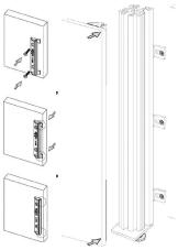
Clip the panel to the first profile, and fix the second profile to the wall.
